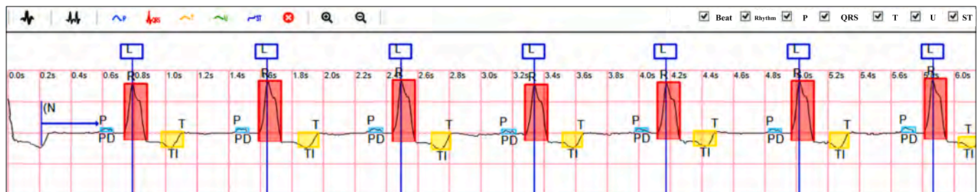
Fig. 1. The image is an annotation interface of the annotation system developed by this paper. The signal in the image is lead I, including beat, rhythm, and morphology labels. Beat annotation interpretation: L → Left bundle branch block beat. Rhythm annotation interpretation: (N → normal sinus rhythm. Morphological annotation interpretation: Above the waveform—P → P Wave; T → T Wave; R → R wave peak, representing QRS wave. Below the waveform—PD → P wave bimodal; TI → T wave inversion.
